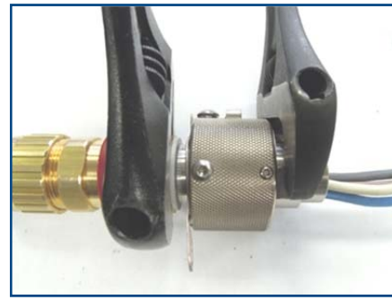
Tighten cable gland to rear shell as shown
